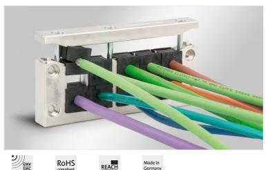
The EMC cable entry frames EMC-KEL-U are based on the KEL-U and KEL-E. Due to a conductive surface, disturbances in the cable shields on the control cabinet can be easily dissipated. Field bound disturbances are derived by the metallisation.
